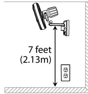
*This fan can only be mounted on an **indoor wall** or on an **enclosed porch** or **enclosed patio wall**.*
