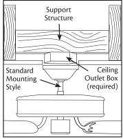
Use **Standard Mounting** to hang the fan from a flat ceiling.
