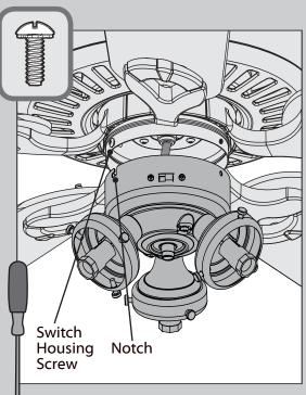
Partially install two of the switch housing screws found in the hardware bag.
