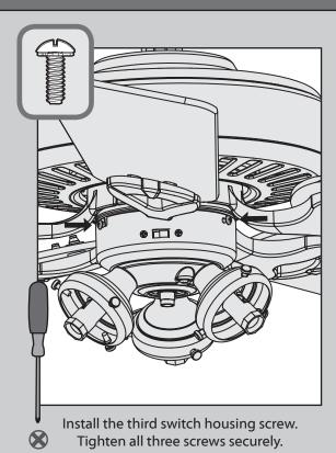
Make sure the lower switch housing is securely attached to the upper switch housing. Failure to properly secure all three assembly screws could result in the light fixture falling.
