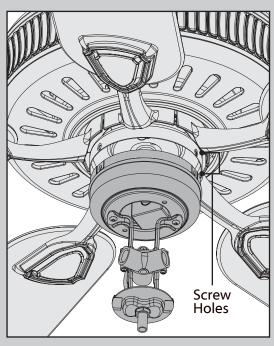
Lift the lower switch housing up until its screw holes are aligned with the screw holes in the upper switch housing.
