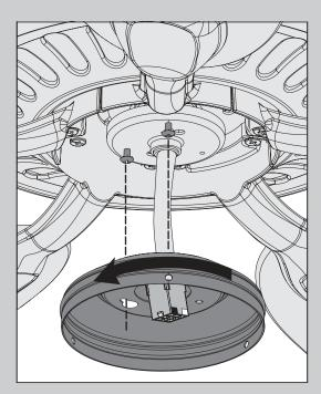
Feed the wire plug through the center hole of the upper switch housing, then wrap keyhole slots around the screws and twist counterclockwise.
