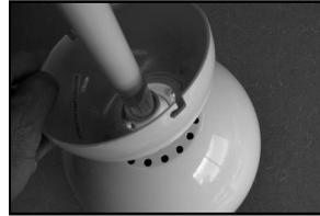
**(7)** Reinstall half ball on end of down rod. Be sure that stopper pin is inserted through down rod and seated in half ball. Tighten set screw against down rod.
