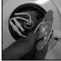
(d) Position all wire leads under socket plate and re-attach plate to fan using screws from step (a).
