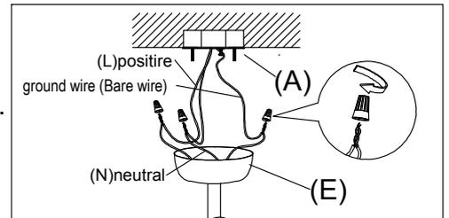
Step.3: Connect the white and black driver wires to the fixture wires with terminal block, connect the white driver wire to the neutral power line wire and the black driver wire to the hot power line wire with wire nuts (see wiring diagram for details). Note: The positive fixture wire is marked by white tracer.
