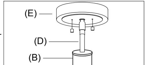
Step.2: Connect the hanger (E) to the lamp body and hook. Determine correct length of rod needed for hanging height. Screw the Rod (D) on the Body (B) and Canopy (E).
